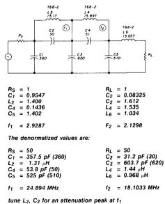
tune L4, C4 for an attenuation peak at  $f_2$
